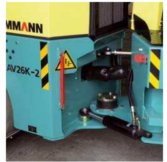
Life time lubricated central articulation joint
