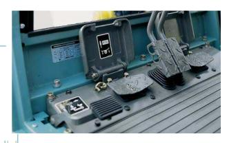
Separated pedals for 3rd circuit and boom swing fitted with robust protections on pedal guards acting as footrests.
