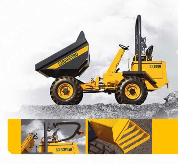
All Barford Dumpers come fitted with a fully certified ROPS safety frame and beacon as standard Thoughtful features such as this all in one secure battery housing and step are inherent in Barford design
