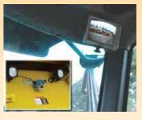
Optional Tyre pressure - monitoring System ensures that the operator has real time information on all tyres pressure and temperature conditions.
