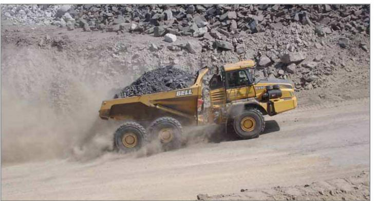
· The exclusive onboard weighing option presents the operator with real time information on the payload while the machine is being loaded. A 'limp home' mode can also be activated if the machine is significantly over-loaded.
