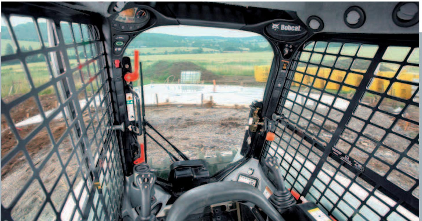
Bobcat new generation loaders have a best-in-class pressurised cab. This features a new one-piece seal that goes all the way around the door and fits into a special curved pocket, keeping dirt and dust out of the operating environment. Sound levels have been decreased by more than 60%, providing improved comfort for the operator.
