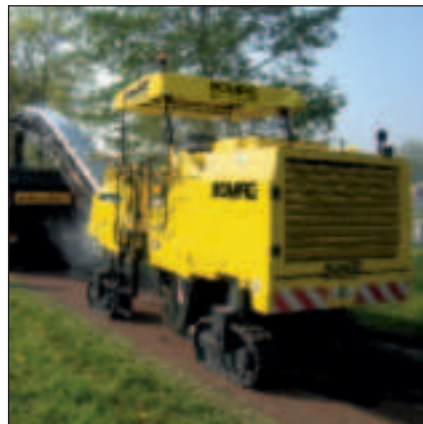
Large crawler tracks prevent sinking on bike or foot paths.
