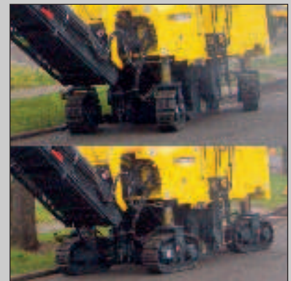
Simple lateral approach to curbs or walls and by-passing of obstructions.
