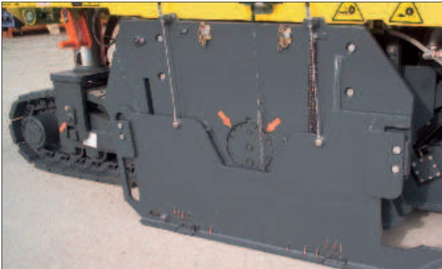
Clearly visible marks for precise incutting. Protected, but still accessible: the cable sensor.
