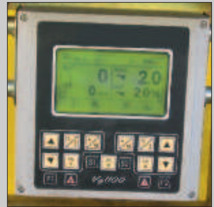
Ready information about machine status, "Intelplaner" automatic milling depth control.
