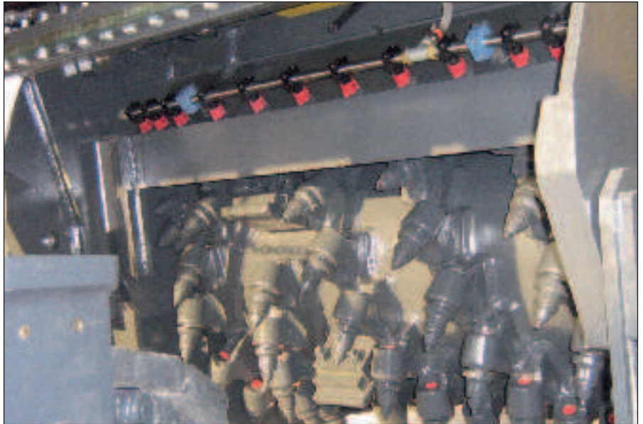
Fast access to milling tools and water bar.
