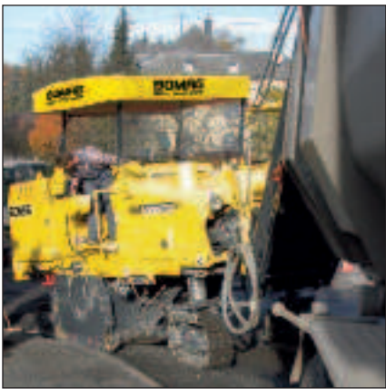
Accurate working without skewing on tight bends with four fully steerable crawler tracks.
