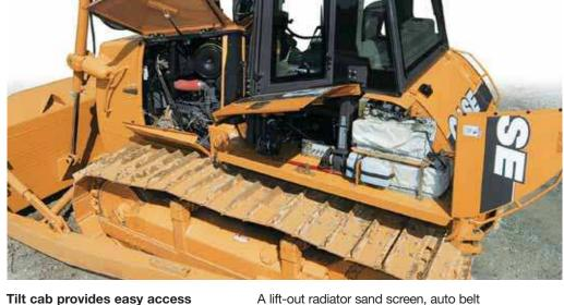
Should your 1650K or 1850K need repair, the operator platform can be tilted in less than 10 minutes to provide convenient access to the for minimized downtime.
