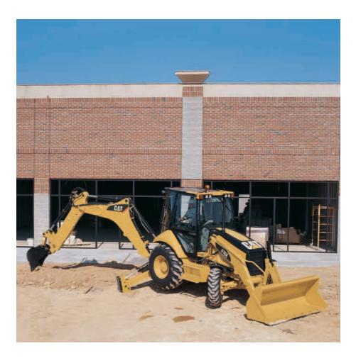
**Flip Over Stabilizer Pads.** Flip over stabilizer pads provide the ability to work in both dirt and street applications. New pads are stronger, feature a positive anti-flip mechanism and provide increased rubber wear life. **Fabricated Grouser Pads.** Designed for dirt applications, the new fabricated grouser pads provide superior strength and durability.
