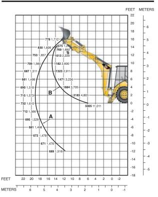
Lift capacities are over-end values. Machine equipped with 4WD, OROPS, 0.76 m<sup>3</sup> (1.0 yd<sup>3</sup>) general purpose bucket, and 116 kg (255 lb) counterweight. Extendible stick includes 488 kg (1,075 lb) counterweight.
