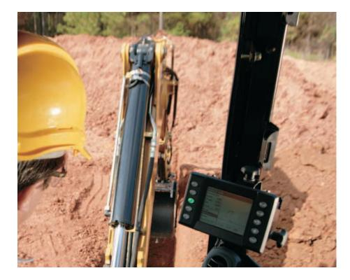
Advantages. Current trenching and excavating processes are labor intensive, dependent on manpower and instruments. Maintaining consistent grade between grade stakes is challenging, even for experienced operators. The AccuGrade® Reference Systems for Backhoe Loaders reduces labor requirements, aids operators in maintaining a consistent slope across the worksite and reduces material cost.
