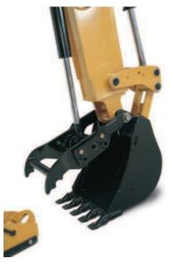
**Thumb Mounting.** Thumb mounting provisions are standard on every Cat Backhoe Loader for added machine versatility. Hydraulic thumbs are available factory-installed.
