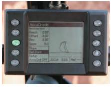
**In-Cab Display.** The AccuGrade monitor allows the operator to enter slope and dig depth parameters. The in-cab display with easy to read grade indicator and elevation display delivers all system information to the cab for easy viewing by the operator.
