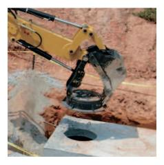
**Thumb.** Available for both the standard and the extendible stick, thumbs increase the versatility of the backhoe with the ability to grip, grab and sort virtually any material.
