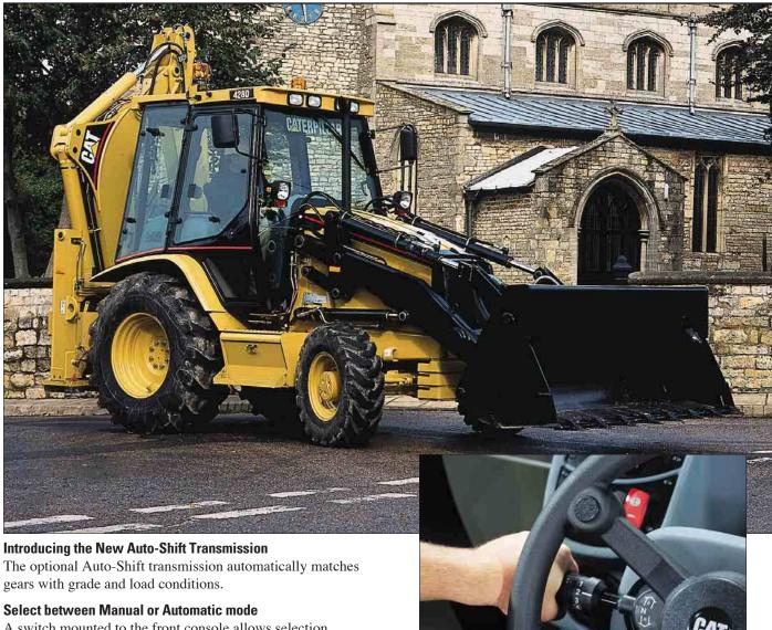
A switch mounted to the front console allows selection between Automatic or Manual mode. In Manual mode, shifting between the gears is achieved by a twist-grip control on the forward-reverse shuttle. Four forward gears and 3 reverse gears are available.
