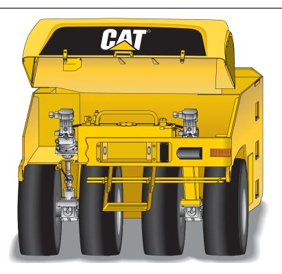
**Hydrostatic transmission** provides smooth direction and speed control, no chains are used.
