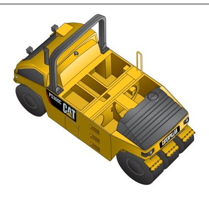
**Maximum operating weight of** 25 000 kg (55,115 lb) provides versatility for thick lifts.
