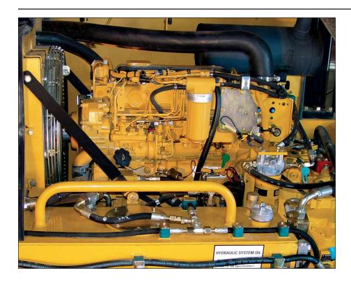
**Turbocharged engine** for top performance and efficiency, even at high altitude with no derating required up to 2134 m (7,000 ft).
