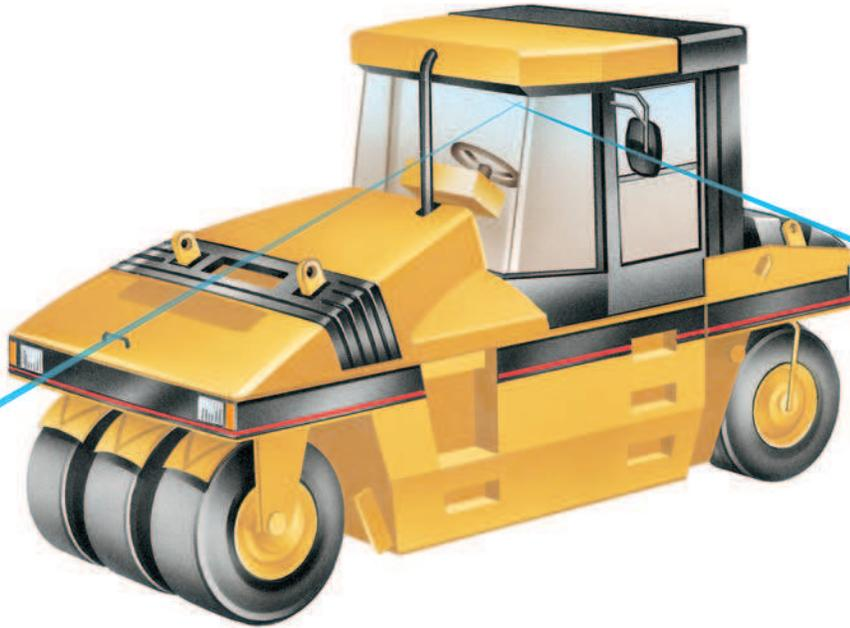
**Visibility.** Excellent forward and rearward visibility allows the operator to see objects 1 meter high and 1 meter in front and rear of the machine.
