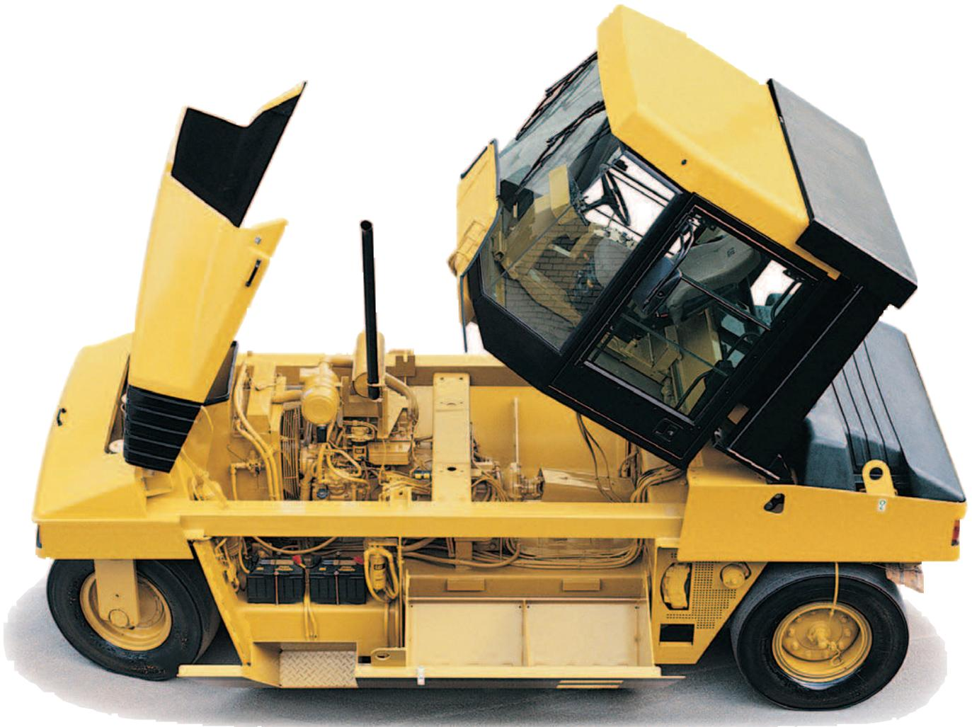
**Routine maintenance points.** They are accessible from engine compartment. Visual indicators allows easy check of radiator coolant, hydraulic oil tank level and air restriction indicator. The engine hood opens quickly with the the use of two gas charged struts to provide unrestricted access to the engine and cooling system.
