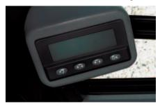
**Messenger.** Messenger is an electronic monitoring system with real-time, visual feedback on engine and machine operating conditions. It provides information on machine performance, fuel consumption, diagnostics, and allows the operator to set some parameters, such as implement and steering modulation.
