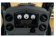
**Instrument Cluster.** The compact instrument cluster (shown with optional AccuGrade GPS display) keeps the operator aware of all vital machine functions. The advanced monitoring system tracks machine operating conditions and informs the operator of impending problems. The monitoring system includes:
