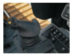
**Bulldozer Control.** The blade is controlled with an ergonomically designed joystick located to the right of the operator. This joystick includes a thumb wheel that controls blade angle. AccuGrade buttons are conveniently located on the joystick for quick, efficient actuation. For non-AccuGrade equipped machines, a blade shake button provides aggressive blade movement for effective removal of sticky material.
