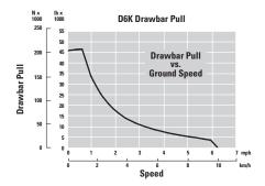
**Torque Rise.** The direct injection electronic fuel system provides a controlled fuel delivery increase as the engine lugs back from rated speed. This results in increased horsepower below rated power. A combination of increased torque rise and maximum horsepower improves response, provides greater drawbar pull and faster dozing cycles.
