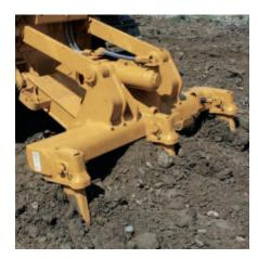
**Parallelogram Ripper.** The multi-shank parallelogram ripper lets you choose one, two or three shanks depending on job conditions. Curved or straight shanks are available. High strength mainframe allows having stiffer ripper mounting blocks for severe drawbar applications. **Drawbar.** The D6K is equipped with a drawbar for pulling work tools such as:
