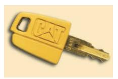
**Cat Machine Security System (MSS).** MSS uses electronically coded keys selected by the customer to limit usage by individuals or time parameters. MSS deters theft, vandalism and unauthorized usage. Each machine system can store up to 255 keys and each key can be used on as many machines as desired. MSS can be controlled by a Personal Data Assistant. Field installation is available.
