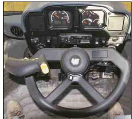
Full machine articulation is accomplished with a  $\pm 70^\circ$  turn of the wheel – versus two to three 360° turns of a conventional steering wheel. The Command Control Steering wheel contains the forward/neutral/reverse switch and the upshift/downshift button – allowing the left hand to remain on the steering wheel at all times. The CCS column inclines 35° and the telescopic change is up to 100 mm.
