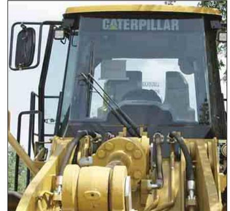
**Cab.** The entire operator station can be removed in about 45 minutes and is easy to re-attach. Quick disconnects are used so no wires need to be cut and no refrigerant is lost. Cab cleaning is made easy with channels on the cab floor and no threshold at the door – the floor can be swept or mopped out easily.
