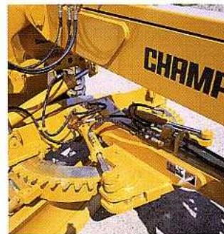
Patented dual-cylinder circle drive uses direct-acting hydraulics for exceptional turning and holding power under full load. DURAMIDE faced clamp plates and guide shoes prevent metal-to-metal contact; and provide longer service life and less maintenance than metallic systems.
