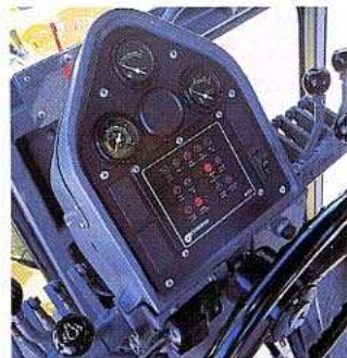
Pedestal includes a 3-level electronic monitor to alert operator to machine status, with backlit switches and fuel level, engine oil pressure and engine coolant temperature gauges.
