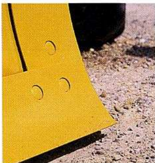
Boron steel cutting edges with 6" bolt spacing. Top and bottom slide rails are supported on DURAMIDE™ bearings, minimizing free play for fine grade control.
