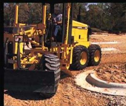
Optimum blade range and a tight turning circle allow Series VI Compact graders to complete a variety of tasks in close quarters.
