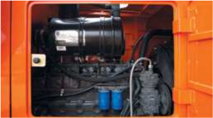
Easy Maintenance Maintenance windows have been added to each side of the engine hood, thus making daily oil inspection and maintenance works quicker and more convenient.
