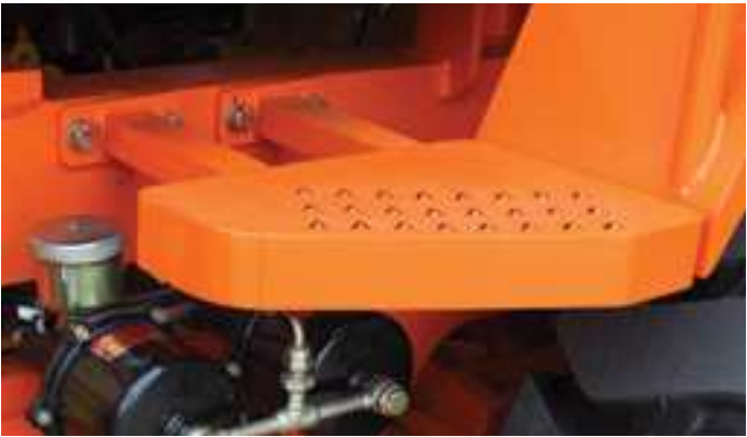
Brake System Check The brake pump is fixed on the side, simplifying routine maintenance work.
