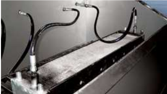
Durability Test Durability tests were carried out to ensure that the radiators work properly under strong pressure fluctuation.
