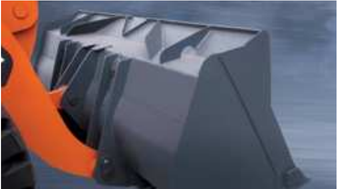
Bucket The bucket is made of high anti-abrasion materials, the bucket's thickness has been increased and a specially designed reinforcing rib has been adopted for the upper part, effectively preventing bucket deformation caused by falling objects such as rocks.
