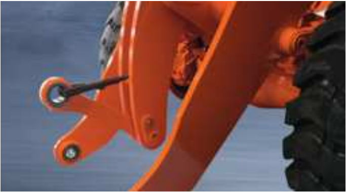
Pin Bushing Pin Bushing is made of high anti-abrasion materials, thus improving resistance to wear and abrasion in the bucket linking positions and prolonging the product's service life.
