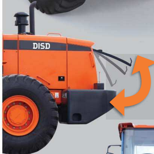
Rear door opening angle increased up to 65°, making engine and radiator maintenance more convenient.
