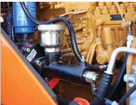
The booster pump delivers a higher augmented-thrust ratio, more stable braking performance, and more convenient daily maintenance thanks to its being mounted on the body's side.
