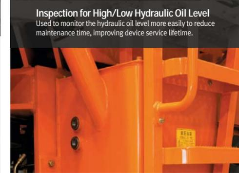
**Inspection for High/Low Hydraulic Oil Level**
