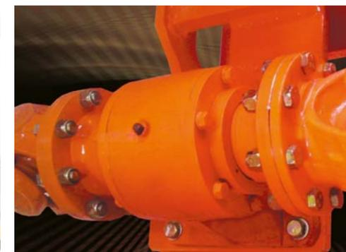
**Transmission Shaft : Double Bearing Drive Shaft**
