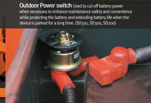
**Outdoor Power switch** Used to cut off battery power when necessary to enhance maintenance safety and convenience while protecting the battery and extending battery life when the device is parked for a long time. (SD310, SD300, SD200)
