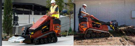
Ideally suited for a variety of demanding jobsites, the Ditch Witch® SK1050 mini skid steer improves versatility and productivity by directing more hydraulic power to the attachment. The durable, construction-grade design eases operator maintenance for improved ROI, and outperforms all other working machines in its class. Designed specifically for the hardworking operator in mind, the best-inclass, spring-supported operator platform improves comfort for long hours on the job.
