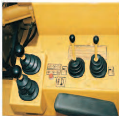
Boom, hook and counterweights controls
