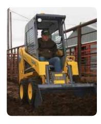
TRANSPORTS EASILY on a small truck or trailer with an overall machine weight of less than 3,000 lbs. (1361 kg), reducing transport costs.
