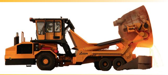
SLV 100 is a special vehicle designed to transport and dump molten slag. It is intended to be used on smooth roadways without greater slopes.
