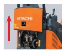
Vertical Sliding Engine Cover Vertical sliding engine cover enables easy maintenance even in confined spaces. When opened, the cover does not interfere with inspection or operation and provides easy access. (Patent pending)
