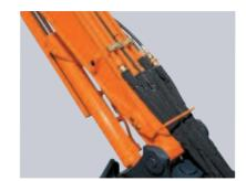
Splitting Front Hose for Easy Maintenance Front hose can be separated on the back of the boom. If the hose
