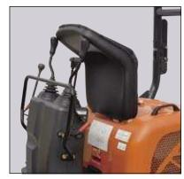
Folding/Retractable Seat Since the seat can be folded up, it can be used immediately after rainy weather, without the need for cleaning.
