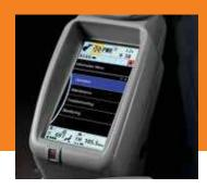
Multi-language LCD monitor and rotary dial provide easy access to machine info and functions. Turn and tap to select work modes, monitor maintenance intervals, check diagnostic codes and set cab temperature. Control oil flow and toggle between dig and thumb modes with a programmable thumb attachment mode.
