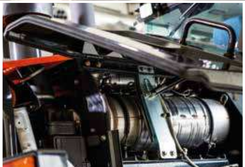
NO DPF SCR system reduces emissions.
