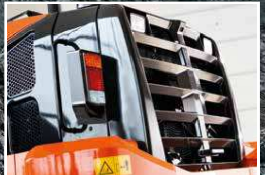
Optional wide fin radiators enhance durability.
