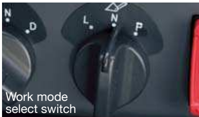
Work mode select switch P mode: Heavy-duty excavation N mode: Loading L mode: Light-duty operation
