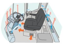
The air conditioner/heater is controlled automatically and thermostatically to enhance operator comfort. Air vents promote good air circulation inside, and defrosting all the year around. The cab is pressurized to keep out dirt.
