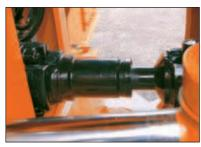
Universal joints are hermetically sealed to extend greasing intervals up to 12 000 hours, simplifying maintenance and increasing durability.
