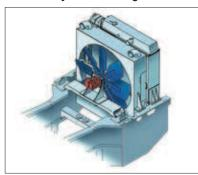
Hydraulic cooling fan speed varies with changes in operating temperatures to reduce noise and fuel consumption. The automatic reversible fan comes standard with a manual override that swings open for easy cleaning of radiators.
