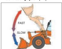
The Efficient Loading System (ELS) can increase traction force during digging while reducing fuel consumption. This achieves more production with less fuel.
