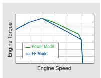
There are two engine modes — Power mode and Fuel-Efficient mode. Select the Power mode to boost power for higher production, and the Fuel-Efficient mode for fuel economy.
