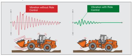
The ride control system can reduce pitching and bouncing when traveling on rough terrain and snow road. This system automatically controls the implement to reduce shocks and vibration.
