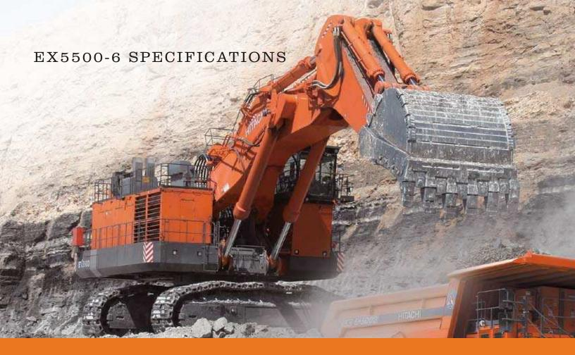
BACKHOE BUCKET CAPACITY: (SAE HEAPED) 38.0 YD.3 (29.0 M3)
