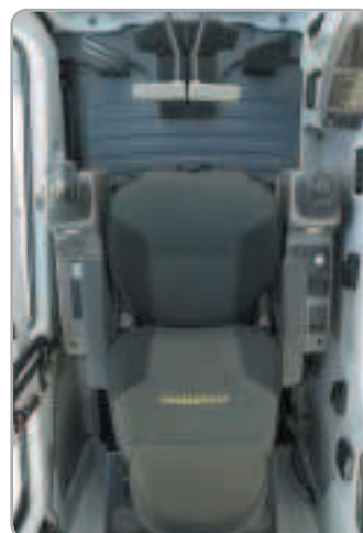
1 2 3 1 Wide, Comfortable Operating Space 2 Steel Cover Sunroof 3 Dial Type Engine Speed Switch and Key Switch
