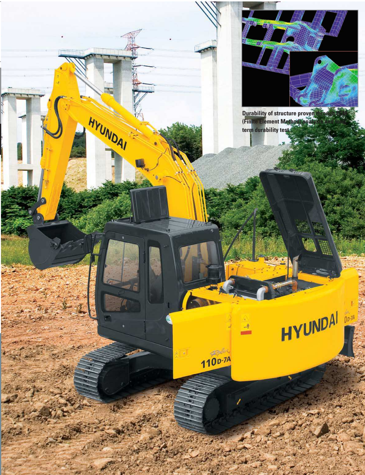
Easy to maintain engine components The cooling and preheating system are provided for optimum and immediate operation, guaranteeing longer life for the engine and hydraulic components. Servicing of the engine and hydraulics is considerably simplified due to total accessibility.
