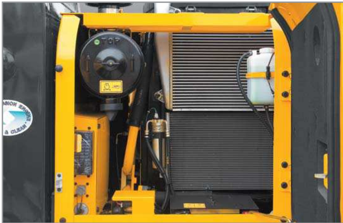
Side Cover with Left & Right Swing Open Type Easy access to vital components gives unrestricted view of component allows easy maintenance and repair.
