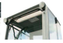
The 15VXT, 16VXT, 17VXT and 19VXT VXT series mini excavators models offer optimum 360° visibility, both for the version with canopy and that with cab, thanks to ample windows. Two adjustable front work lights, protected to prevent accidental breakage, allow the operator to make use of optimum lighting of the work area. Boom geometries offer excellent digging performance down to a depth of 2460 mm.
