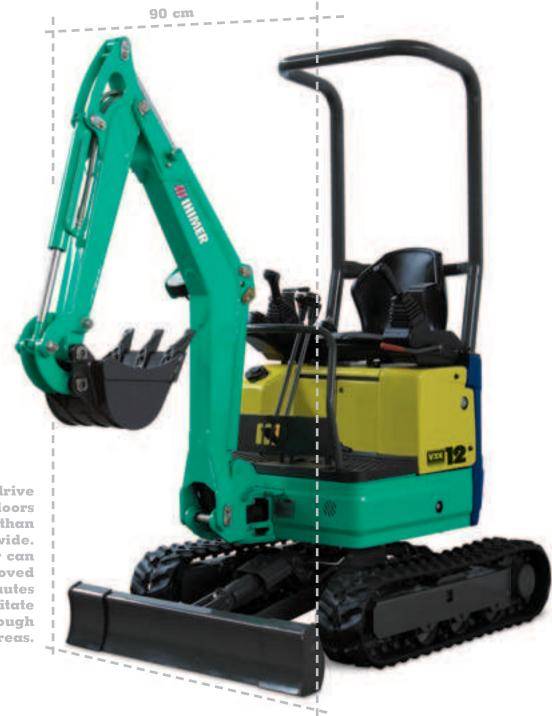
The 12VXE can drive through doors no more than 90 cm wide. The rollbar can also be removed in just a few minutes to facilitate passing through low clearance areas.
