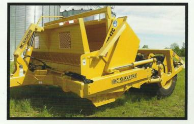
The Carry All Dump series scraper is used for soil transport & precision leveling. It has a gate for transporting material and a bowl that pivots then dumps the material where needed. The reinforced frame is designed to comply with higher horse powered tractors and heavier load capacities.
