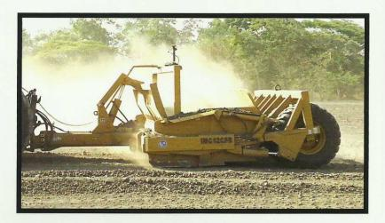
The CFB has a reinforced frame, tongue, and carriage designed to comply with higher horse powered tractors and heavier load capacities.
