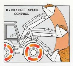
• Hydraulic Speed Control either. channels all the hydraulic flow to the loader for fast speed operation or it returns flow back to the tank.. This releases greater engine power to the transmission, and allows easier and more precise loader control.
