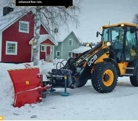
With our High Flow option, you get an extra 30 litres of hydraulic capacity for an
