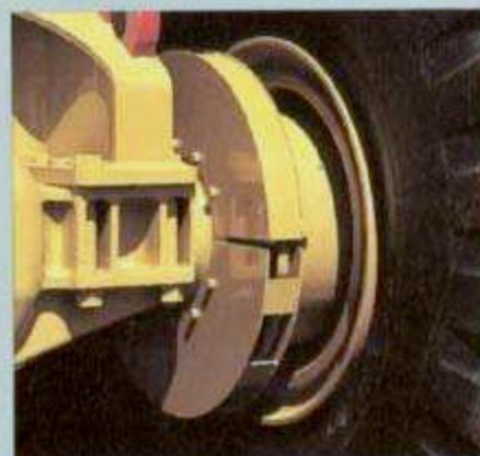
adjusting. The brake pads have electronic sensors to monitor wear. Easy to service in the field, the new pads can be installed quickly. The front and rear axles have separate systems for added safety. The emergency brake automatically applies in case of pressure loss.
