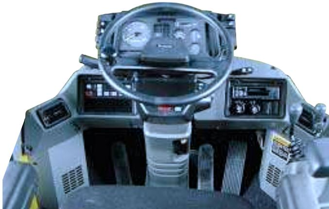
*Easy-to-read gauges and adjustable tilt-ster with attached instrument panel provide accurate information at a glance.*
