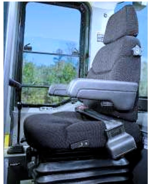
*The bucket seat with adjustable armrests and headrest is fully adjustable, providing comfort, visibility and accessibility to levers, pedals and displays.*
