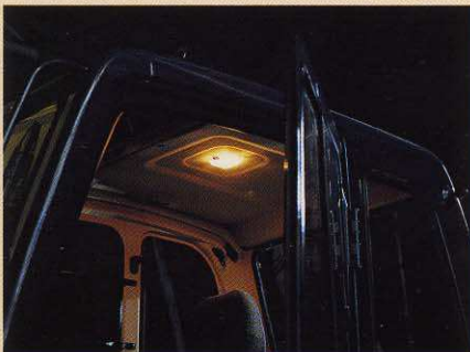
Cab interior light activated by opening the door makes nighttime mounting and dismounting safer.
