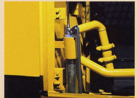
Grease gun holder is always close to hand, stowed just inside the engine guard.
