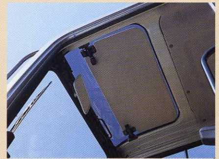
Sun visor to reduce the glare of the midday sun, with a stowing support.
