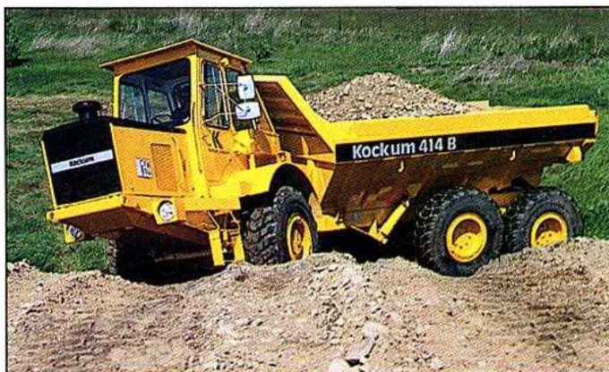
Suspension, 6-wheel drive, triangular design bogie, lock-up and fully enclosed multipledisc brakes give the Kockum 414B unique driving characteristics on difficult surfaces.
