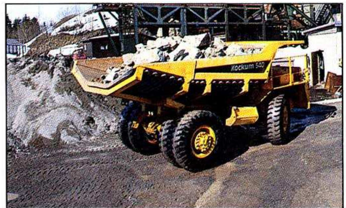
The Kockum 540 can be equipped with a special body with rubber bottom (Rubber Body), which increases load efficiency and also considerably reduces the sound level when loading and unloading.
