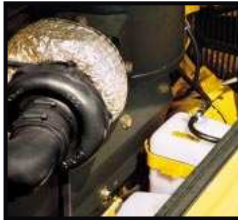
A radiator coolant reservoir makes it easier to check the coolant level and eliminates frequent refilling.
