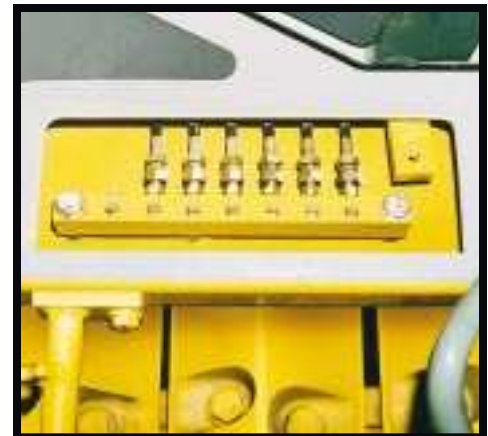
Oil pressure test ports for the power train are centralized on the right hand side of the operator platform for easy access.
