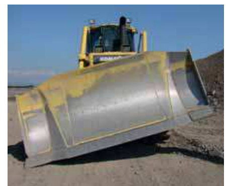
Hydraulically adjustable tilt: 870 mm
