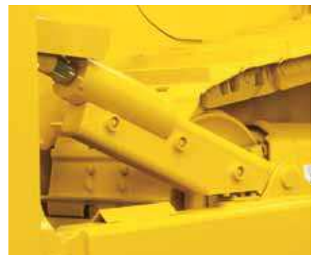
Hydraulic lines are embedded into the structures whenever possible
