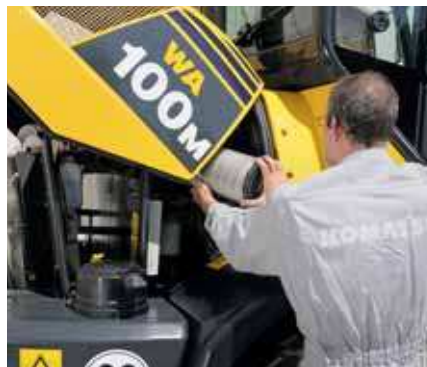
Convenient air filter access
