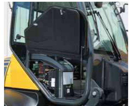
Side cover for quick maintenance access
