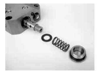
11) Remove the plug (V11), and then remove the spring (V9), washer (V13) and spool (V7).Do not use spanner but use socket wrench.
