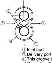
③ This groove is inlet side.④ Gear side sliding face
