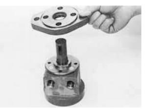
(9) Mount flange into housing saay. Care should be taken not to damage seal with shaft key.
