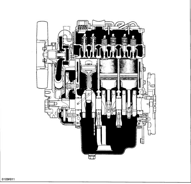
The Z442-B, Z482-B, D662-B, D722-B are vertical, liquid-cooled, 4-cycle diesel engines.
