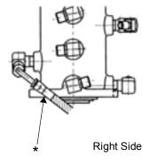
\* Center of metal fittings of hose should be located at same line of bottom of Rotary joint.
