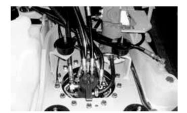
2) Connection of the hose (return 2) Tightening torque of hose clamp (10-22): 2.9 ~ 3.9 N·m (3.0 ~ 4.0 kgf·m)
