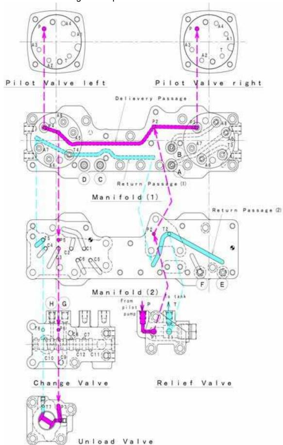
a. Control lever lock being at lock position
