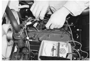
Is voltage applied for about 10 sec. when the starter switch is OFF? (Photo 3)
