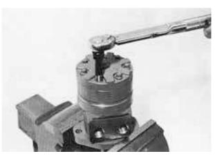
(2) Remove 7 pieces of end cap bolts and seal washer.When mounting on vice, clamp at flange part not, not housing.
