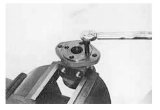
(11) Mount the motor housing by vise as shown in photo, remove 4 pieces of flange mounting bolts.
