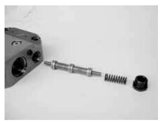
2) Mount the orifice plate (V23), spring (V21) and pilot poppet (V20), and tighten the plug (V19) with specified tightening torque.
