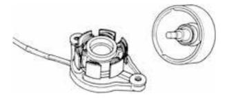
This AC dynamo is so designed as to mount a cooling fan at the shaft end and composed of a rotor and stator.
