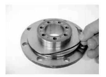
11) Mount the parallel pin (16) to the valve (19). (2 locations)
