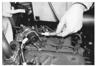
Apply battery voltage to the engine stop solenoid and check to see whether or not the injection rubber is drawn in and the rack bar returns when the application of voltage is stopped. (Photo 5)
