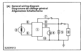
This dynamo is an 8-8 pole rotating magnet type generator. It is simple in construction, consisting of a stator and rotor. The rotor is made up of eight permanent magnet pole pieces assembled on a shaft and rotates on the center of the stator around which eight electromagnetic coils are provided for. This dynamo produces higher voltage in slow speed rotation, and charges electric current to the battery during engine idling.
