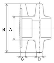
(A)New machine reference value (B)Allowable limit
