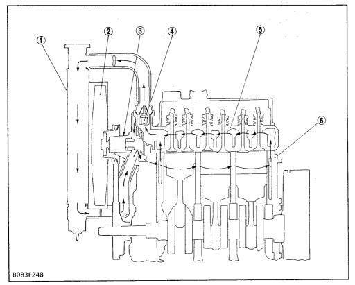
The cooling system consists of a radiator (1) (not included in the basic engine), centrifugal water pump (4), suction fan (2) and thermostat (3).
