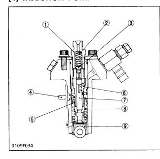
A Bosch MD type mini pump is used for the injection pump. It is small, lightweight and easy to handle.
