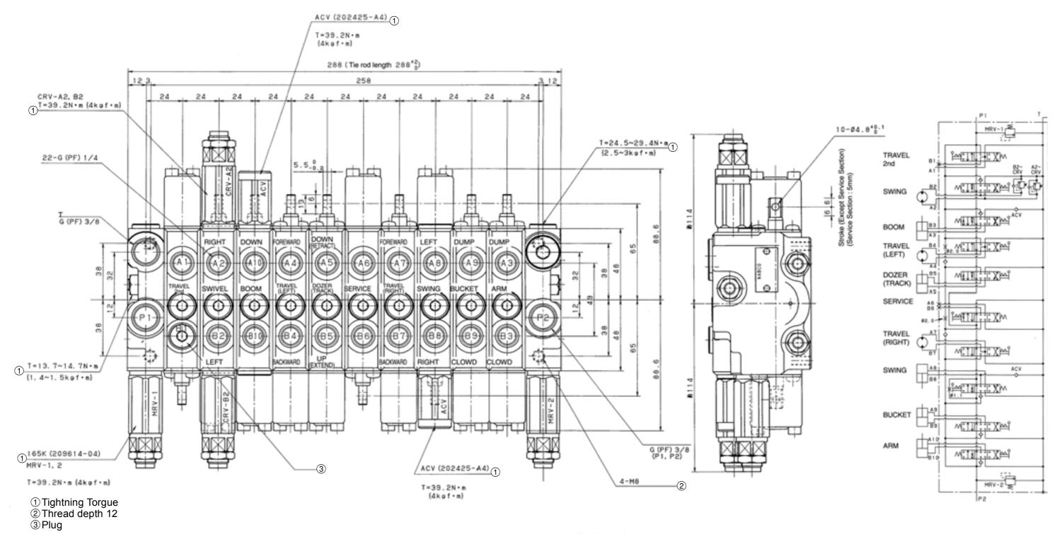
MRV=Main relief valve CRV=Overload relief valve ACV=Antiboid valve
