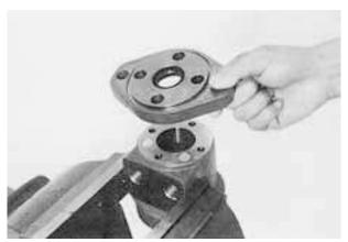
(12) Take out flange. In case of S-280 and S-380, 4 pieces of spring pins are installed, Therefore, remove flange by slightly topping the flange by plastic hammer, then pull out spring pins.
