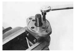
(10)Clamp at housing with vise and tighten 4 bolts. (Tightening torque 25.5 ~ 31.4N·m (2.6 ~ 3.2kg·m))
