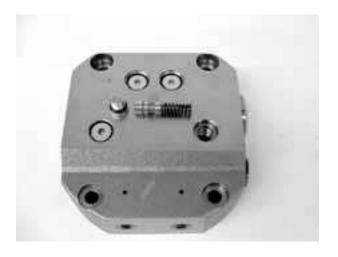
15) Remove the plug (V19), and then remove the pilot poppet (V20), spring (V21) and orifice plate (V23). Use care not to confuse right and left combination of the pilot poppets.This procedure is not needed for TRBF (1-speed motor).
