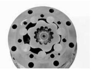
14) Mount the valve plate (17). Phase position can be aligned by matching with the wheel hole. Put a mark by felt pen to the same phase position as the position where the valve is marked.
