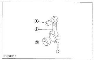
The crankshaft with the connecting rod converts the reciprocating motion of the piston into the rotating motion.
