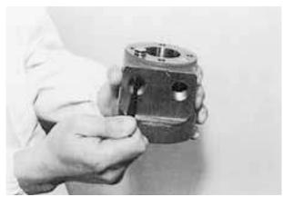
(17) Take out two plugs from housing. Inserting throush port hole, push up the plugs. If not in need, never remove check plug.
