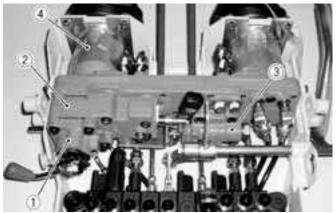
(1)Unload valve Unload valve assembly drawing
