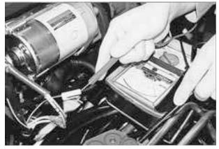
Is battery voltage applied to the self-starting motor in starter switch ON position? (Photo 4)
