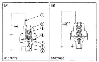
The oil pressure switch is mounted on the cylinder block and is led to the lubricating oil passage.
