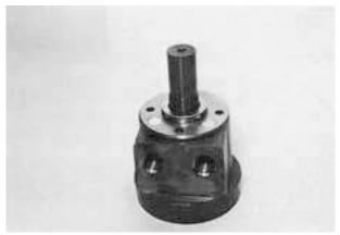
(3) Install output shaft in housing.
