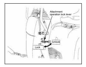
When air enters the hose for pilot valve or the manifold, the attachment may not be operated even when the engine is started and the operating lever is manipulated.
