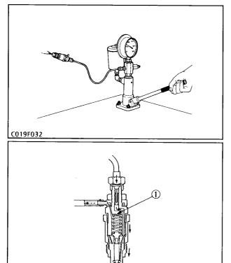
**Checking Nozzle Injection Pressure**
