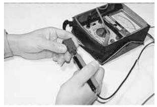
1. Checking slow-low fuse for breakage (Photo 3)
