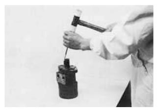
Tap out shaft key. Remove bur around shaft key groove by using sand paper or oil stone.
