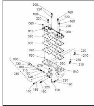
Valve assembly (Relief) structural drawing
