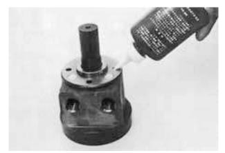
(8) Thoroughly clean flange mounting screw holes of housing, remove grease and apply screw-locktite slightly. (S-280 and S-380 dose not require this job.)
