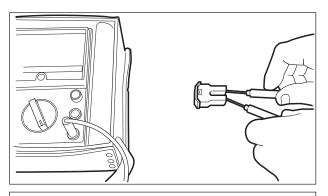
Case where fuse is blown by overcurrent
