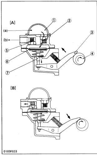
The filtered fuel is fed to the injection pump by the fuel fed pump.
