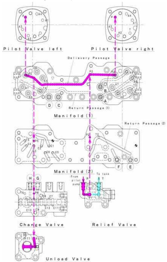
b. Control lever lock being at unlock position
