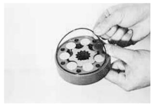
(14 Fit O-ring (2 pieces) onto geroler. Apply grease on O-ring and securely fit.
