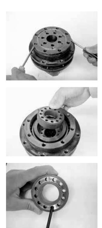
6) Dismount the valve plate (17) by inserting a screwdriver between the valve plate (17) and the wheel (10).
