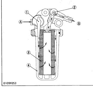
Each moving part of the injection pump and nozzle is extremely precision machined, and clearances of their sliding parts are extremely small. Fuel itself serves as lubricating oil. For this reason, it is extremely important to completely remove water and dirt contained in fuel.
