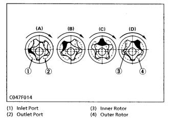
The oil pump is a trochoid pump, whose rotors have trochoid lobes. The inner rotor (3) has 4 lobes and the outer rotor (4) has 5 lobes, and they are eccentrically engaged with each other. The inner rotor, which is driven by the crankshaft through the gears, rotates the outer rotor in the same direction, varying the space between the lobes.
