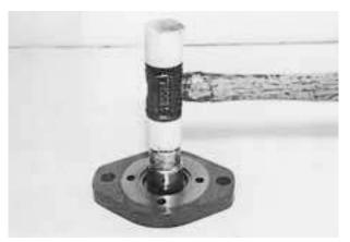
When press fit the dust seal and oil seal, use socket ans tap in with hammer.
