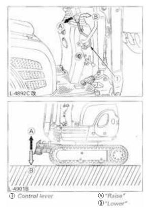
2. While undertaking earth moving work, control both drive levers with the left hand and the control lever with the right hand.
