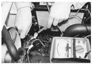
Check conductivity between the solenoid terminal and the body ground. (Photo 6)
