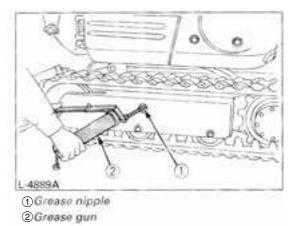
2. Tension the crawler in the lifted position, so that the distance "A" (clearance between the track roler and the inside surface of the crawler) is 10
