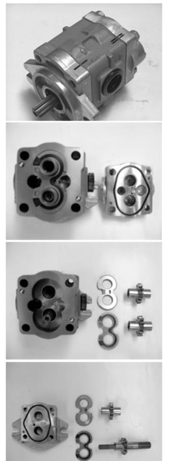
(1) Before disassemble, put alignment mark on front cover, body and rear cover and remove bolts.
