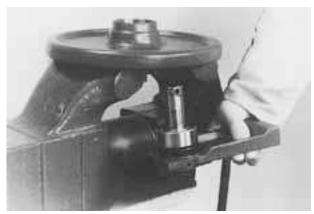
3) Remove the plate and dismount the idler support by gear puller.
