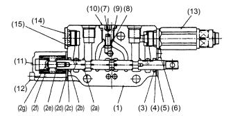
For smooth movement and easy inching adjustment of the spool, the passages of the hydraulic source, working section and tank are all inter connected while the spool is switched over.
