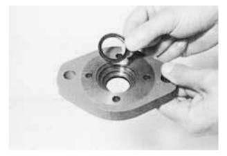
(5) Install oil seal in flange as shown in Fig.
