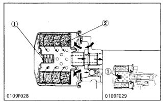
The relief valve prevents the damage to the lubricating system due to the high pressure of the oil.
