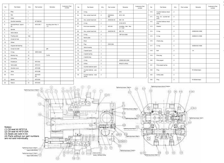
[5] Wheel motor component parts
