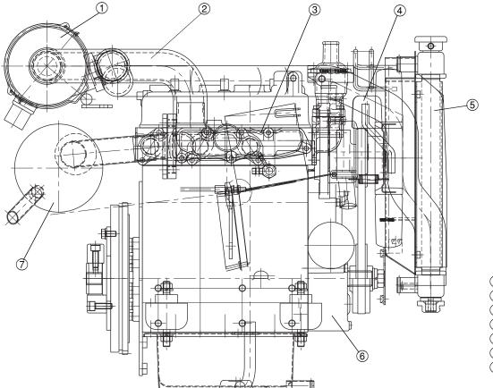
① Starter moter 2 Alternator3 Accelerator cable
