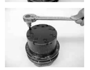
19) Tighten eight M10 bolts (24) and seven M8 bolts.Tightening torque M8: 3 kgf·m M10: 5.7 kgf·m
