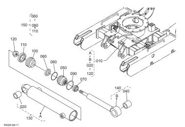
Track cylinder and component parts
