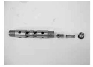
13) Remove the orifice (16) which is fitted to the housing.
