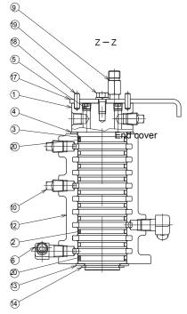
Swivel joint's adaptor mounting angle should be within the range shown in the drawing.
