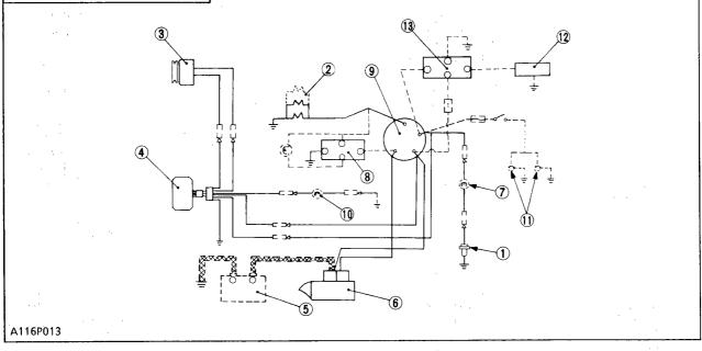
The electrical system of the engine consists of a starting system (including a starter, glow plugs and others), a charging system (including an AC dynamo, a regulator and others), a battery and an oil switch.
