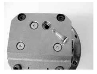
Put in the ball (V18) and tighten the check plug (V16) with specified tightening torque.
