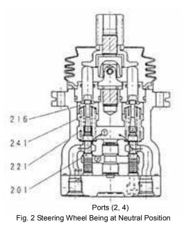
2) When the steering wheel is inclined (See Fig. 3.) When the steering wheel is inclined to stroke the push rod (212), the (spring seat (216)) spool (201) moves downward, the P port communicates with the ports (2, 4) and oil supplied from the pilot pump flows to the ports (2, 4) to generate pressure.
