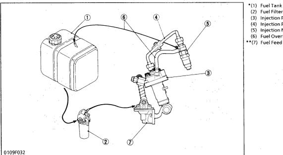
(2) Fuel Filter (3) Injection Pump (4) Injection Pipe (5) Injection Nozzle (6) Fuel Overflow Pipe \*\*(7) Fuel Feed Pump
