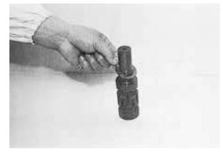
(10) Take out needle bearing from output shaft.
