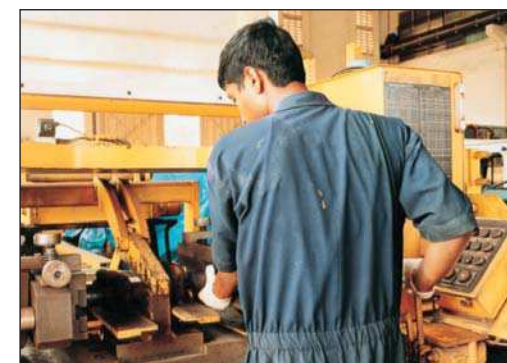
Track chain re-assembling using track press
