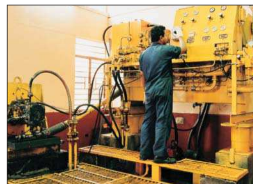
Checking the valve block at Hydraulic Test Bench
