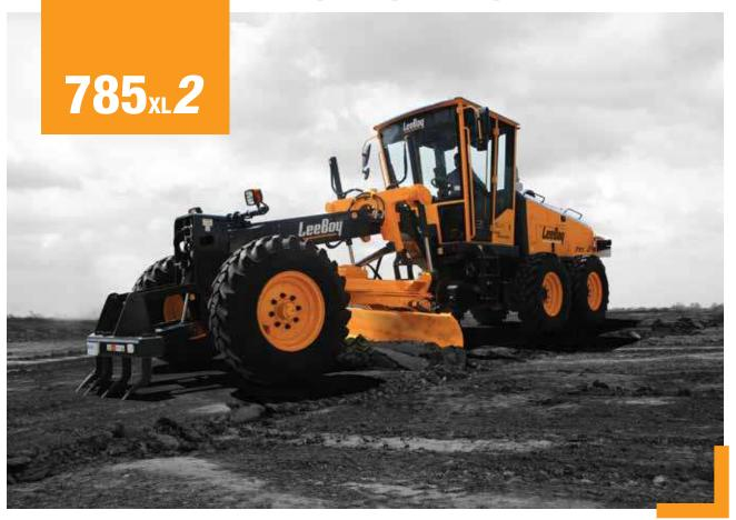
CUMMINS 6BTAA5.9 - 150 C | SIX-FORWARD, THREE REVERSE, AUTOMATIC POWER SHIFT TRANSMISSION | NO-SPIN DIFFERENTIAL TANDEM AXLE | OPERATING WEIGHT 13,200 KG 12-FEET MOLDBOARD | ERGONOMICALLY DESIGNED CABIN WITH HVAC AND EXCELLENT VISIBILITY | CENTRALIZED ELECTRONIC DISPLAY
