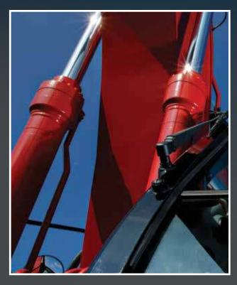
Greater digging power and increased lift capacities are the result of our innovative Spool Stroke Control (SSC) system, which reduces pressure loss and distributes hydraulic oil more smoothly. Pilot pressure sensors detect the type of work being done-such as digging or leveling-and then relays that data to proportional solenoid valves that quickly determine where optimal hydraulic pressures should be directed for that operation.
