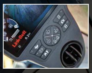
High-Definition LCD monitor has a full-color 7" display that rivals the resolution found in luxury automobiles. Controls are easy to read and easy to use. The rearview camera activates automatically whenever the machine is started, and sight guidelines have been added for increased safety.
