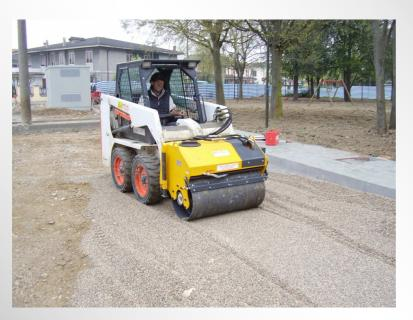
PRECISION THANKS TO ITS SHAPE AND SIZE IT ALLOWS GOOD VISIBILITY TO WORK WITH ACCURACY. THE ROLLER HYDRAULIC DRIVES ARE SAFETY PROTECTED. THE DRUM ROLLER STEEL SCRAPER BLADE ENSURES SMOOTH AND UNIFORM COMPACTION PERFORMANCES.
